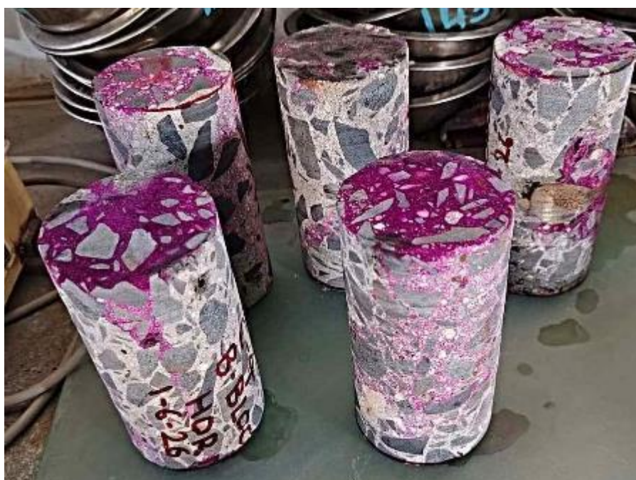
Carbonation Test on Core
