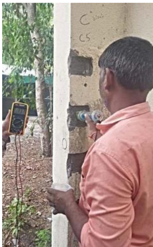
Half Cell Potential Test
