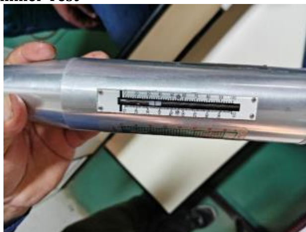
Rebound Hammer Test
